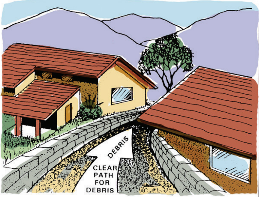
Figure 6: Directing Debris Flows Between Buildings – How to channel debris through and away from buildings.
