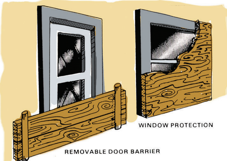
Figure 14: Typical Window/Door Protection – Use of plywood or timbers can help protect windows and doors from damage.
